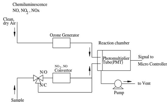
Measurement of  $\text{NO}_x$  is accomplished by means of a catalytic converter, which converts  $\text{NO}_2$  to NO prior to reaction with ozone. The ozone required for the reaction is generated internally within the instrument.
