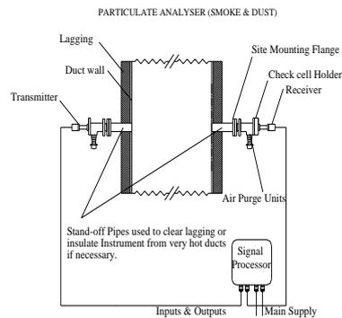
The amount by which it is reduced being a function of the particulate loading of the gas. These instruments use a motor and notched blade to physically “chop” the light beam. The light source can be modulated electronically. The detector and detection circuitry are designed to be sensitive only to light with the precise frequency and phase.
