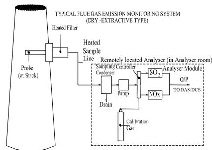
This system removes moisture through a combination of refrigeration, condensation and permeation tube dryers that pass the sample through water excluding membranes. This system helps keep the gas analyser dry and removes any interferences caused by water. Calculation of moisture removed adds complexity to the system. Operating an extractive system is complicated by the daily calibration, zero and span checks of the analysers
