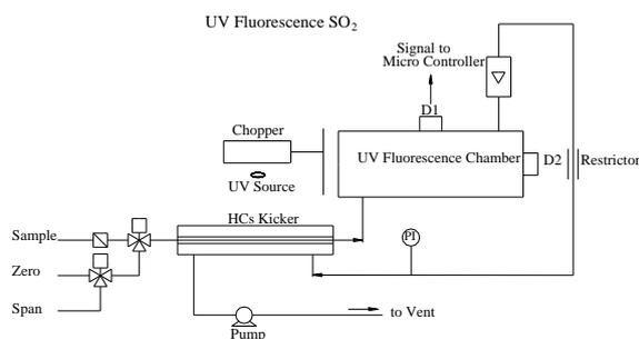
The UV light is chopped, filtered and focused into the fluorescence chamber where it excites the SO<sub>2</sub> molecules into a higher energy state. As this energy decays the excited SO<sub>2</sub> modules emit a characteristic radiation. A second filter allows only radiation at the characteristic wavelength to reach the photomultiplier tube (D1), which converts the radiation into electrical impulses. These impulses are filtered, amplified and scaled
