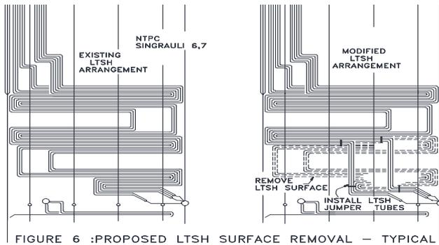
FIGURE 6 :PROPOSED LTSH SURFACE REMOVAL – TYPICAL
