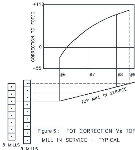
Figure 5 : FOT CORRECTION Vs TOP MILL IN SERVICE - TYPICAL
