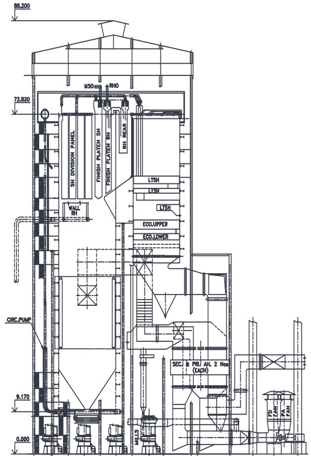
**FIGURE 1: GENERAL ARRANGEMENT OF BOILER – TYPICAL**
