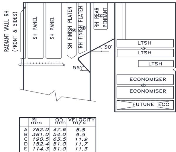
**FIGURE 2: PRESSURE PART ARRANGEMENT—TYPICAL**
