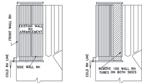
FIGURE 7 : PROPOSED WALL RH SURFACE REMOVAL – TYPICAL
