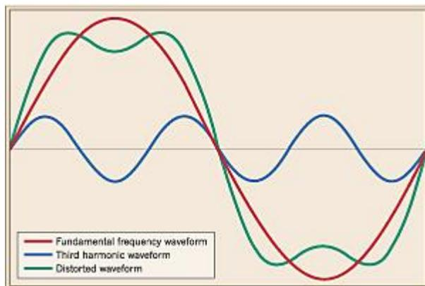
Harmonics Distortion in voltage and current in any electrical system leads to;
