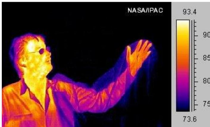
Image with infrared camera. See the colour pattern and temperature profile. (Courtesy: Wikipedia)
