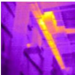
Thermogram of overheated bus bar.
