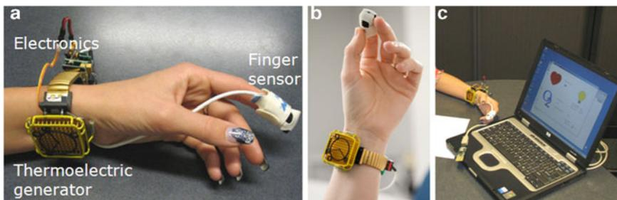
**Fig. 2.9** Wireless pulse oximeter (a, b) and the application running on a laptop (c)
