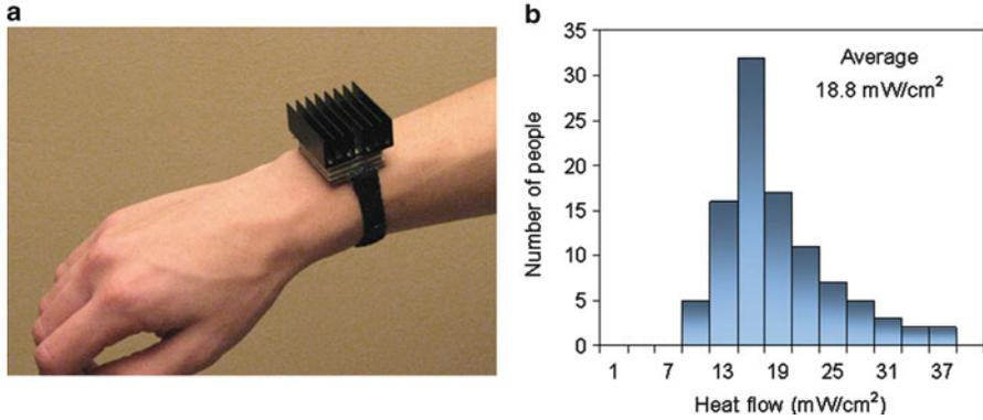
**Fig. 2.6** (a) Thermoelectric generator on the wrist and (b) the heat flow through the TEG per square centimeter of the skin measured indoors on the wrist of 100 people sitting still at a mean room temperature of 22.3°C
