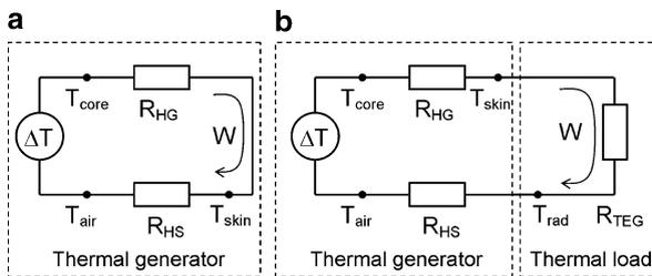
**Fig. 2.1** Equivalent thermal circuits of: (a) a short-circuit natural thermal generator, and (b) the same generator with a thermal load. A relatively small surface of the skin, e.g., several square centimeters, is considered in both cases for the sake of simplicity
