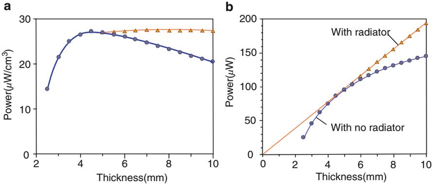
**Fig. 2.4** Calculated dependence of the power on a thickness of an optimal TEG with no radiator (circles) (Fig. 2.2b), and with the radiator of an optimal size (triangles) (Fig. 2.2c): (a) power per unit volume, (b) power produced in a TEG of 3 cm in diameter. A dashed line in (b) is the guide for an eye
