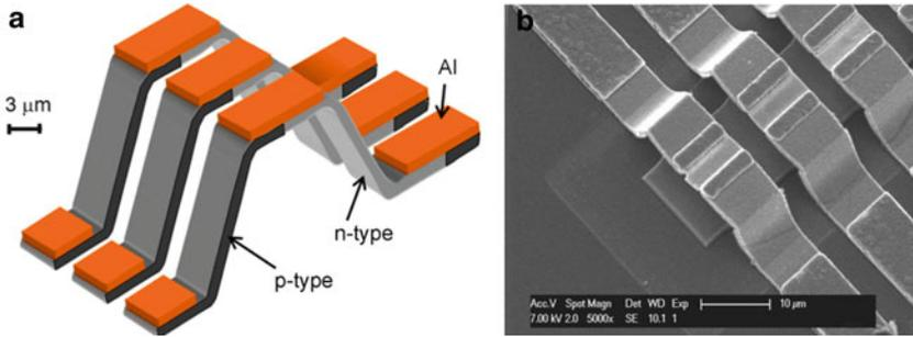
**Fig. 2.14** Surface micromachined arcade thermopile. (a) The conceptual design of a thermocouple. Three thermocouples are shown. (b) An SEM picture of a poly-SiGe thermopile test structure with a 6  $\mu\text{m}$  topography and a critical dimension of 3  $\mu\text{m}$  (reproduced from Su et al. 2010 with permission from Elsevier)
