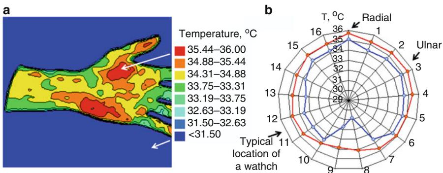
**Fig. 2.5** (a) Temperature map of the hand (palmar view). The infrared image is taken with calibrated radiometric camera within the 8–12  $\mu\text{m}$  spectral range. (b) Temperature profiles around the wrist with a circumference of 17 cm at two ambient temperatures, 27°C (circles) and 22.3°C (diamonds), measured indoors
