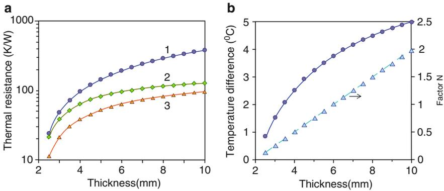
**Fig. 2.3** Calculated dependence of thermal characteristics of optimal both the thermoelectric generator and the thermopile on the thickness of a TEG: (a) the optimal thermal resistance of an empty TEG (1), of the matched TEG (2) and of the thermopile (3), and (b) the temperature difference on a thermopile (1) and the factor  $N$  (2)
