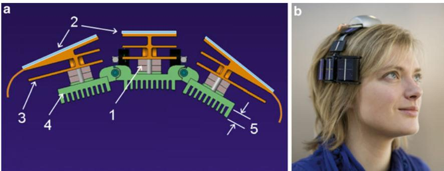
**Fig. 2.11** (a) Cross-section of the hybrid thermoelectric-photovoltaic generator unit used in an EEG system: (1) is a thermopile, (2) are PV cells, (3) is a radiator, (4) is a hot plate with (5) thermal shunts. (b) Two-channel EEG system with a hybrid power supply (reproduced with permission from Van Bavel et al. 2008)
