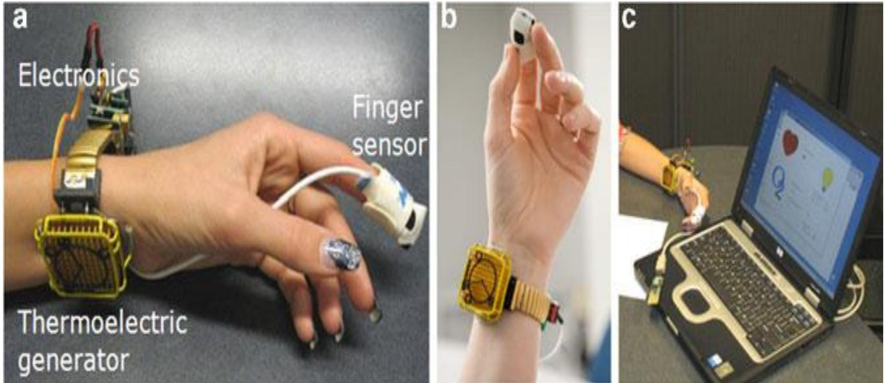
**Body powered pulse oxymeter**
