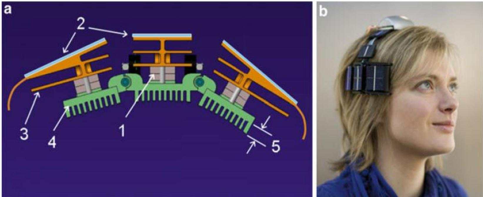
a) Cross section of Hybrid power source for EEG
