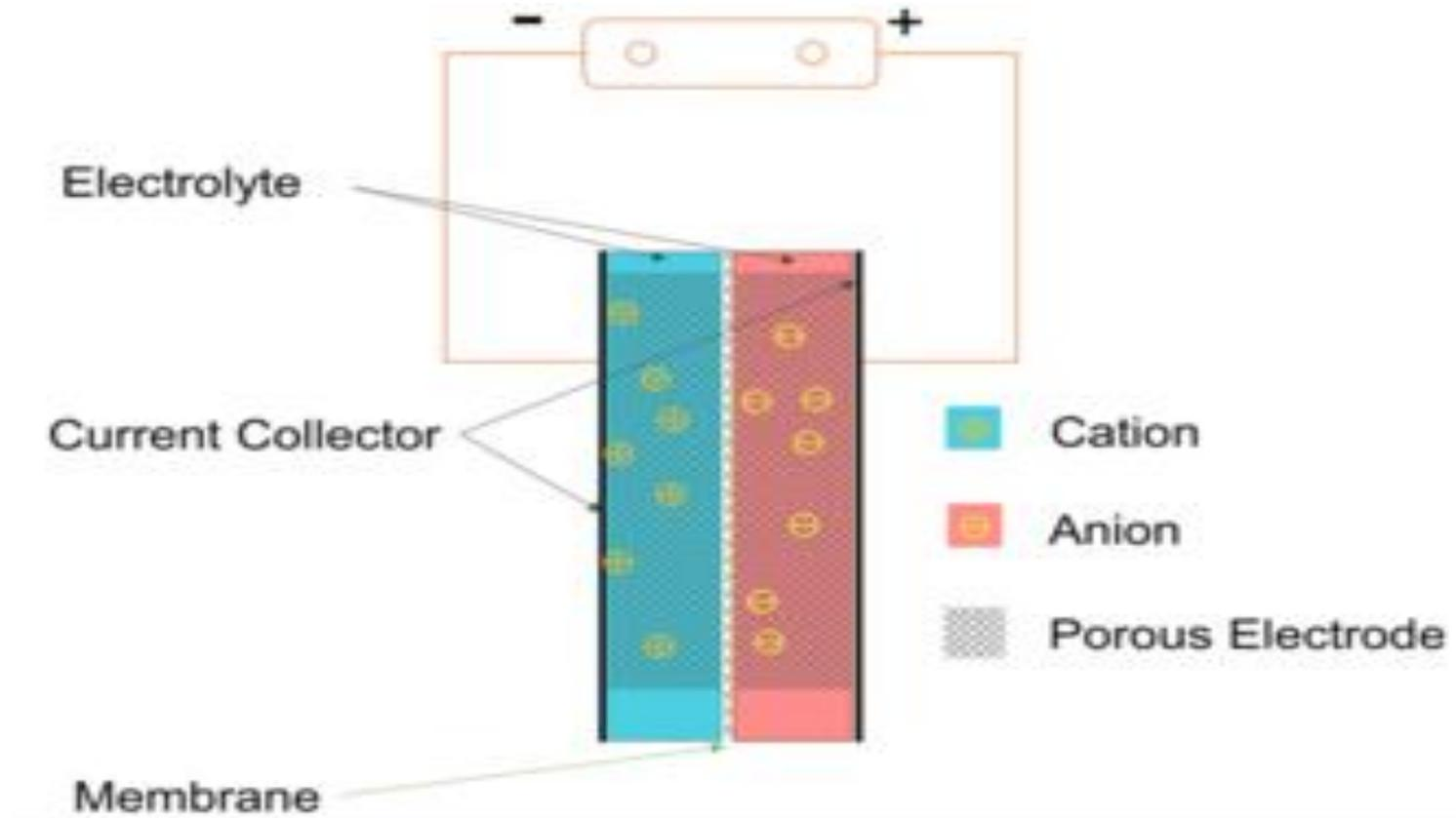
Super capacitor or ultra capacitor is high capacitor with lower voltage limits
