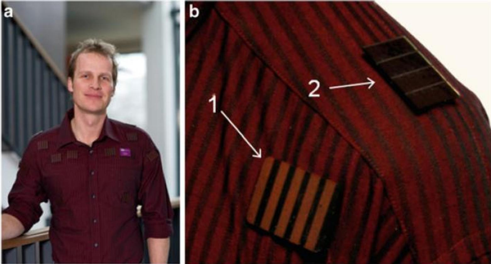
a) ECG system integrated in a shirt    b) Thermo electric module (1) and PV cells(2)
