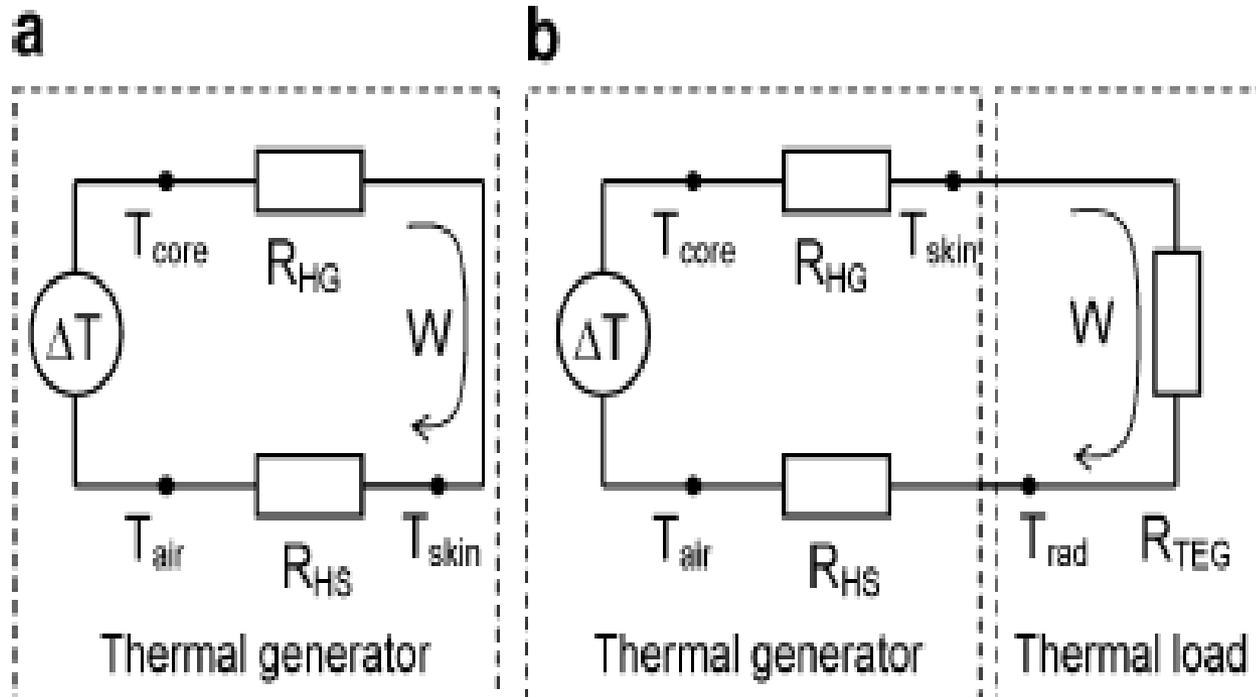
Thermal equivalent circuit
